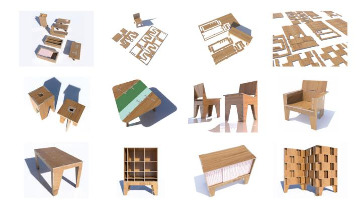
**Process:** CNC Router (subtractive fabrication)
