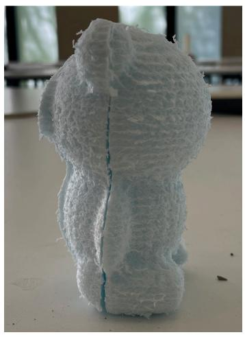
**Process:** CNC Router (subtractive fabrication)
