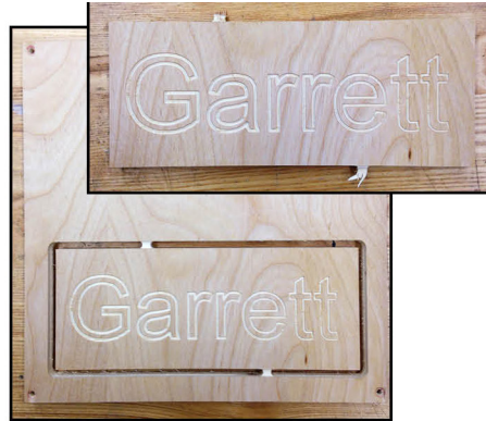
3. Removed from Router & Popped Out Bridges
