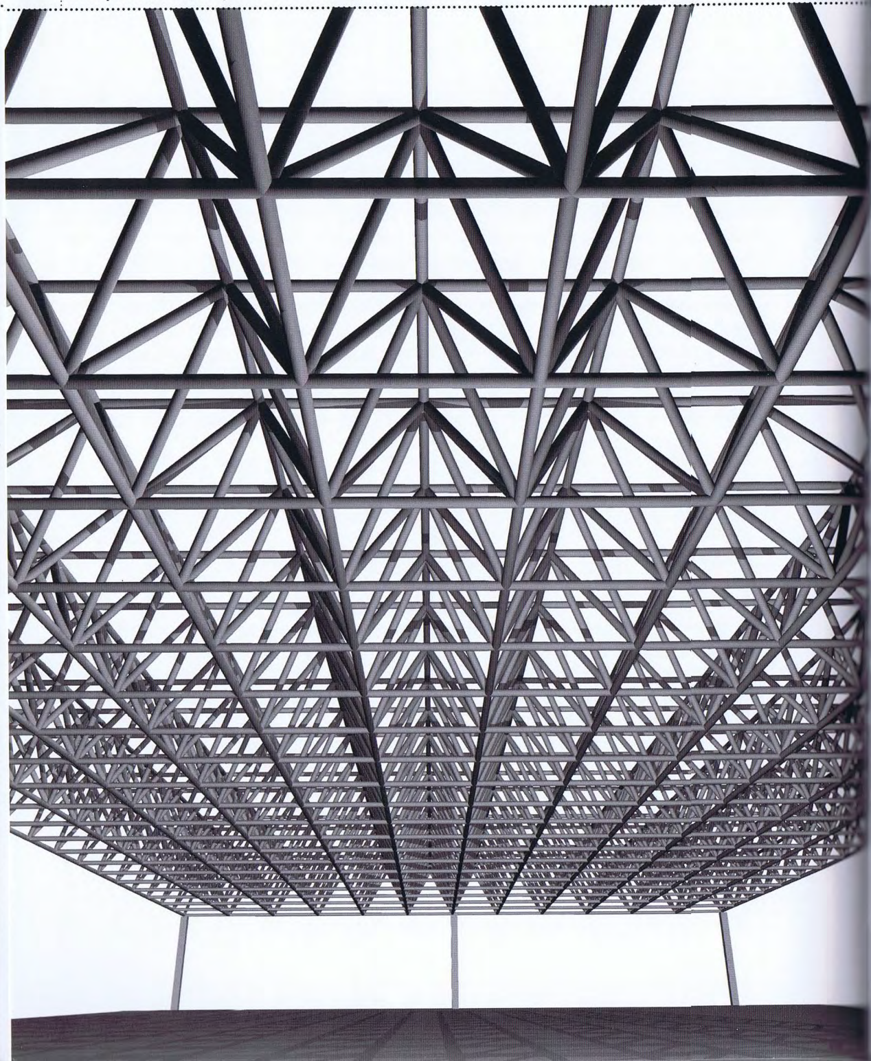
This horizontal form is produced by the tessellation of a base unit composed of a double grid of struts, tubular in section, which are interconnected by diagonal struts. The base unit simply repeats, but its depth and scale can vary, altering the rigidity and porosity of the structure. The struts can also be distributed regularly or irregularly along the double-layer grid to connect them at right angles or diagonally. This assembly transmits an optical affect of repetition, openness and lightness, and an acoustical affect of diffusion and specularity.
