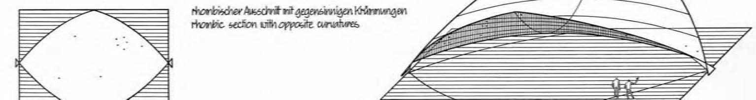
torus sections for special plan geometry
