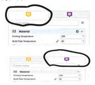
THE FILAMENT THAT WE PRINT WITH, USES THE DEFAULT SETTINGS FOR TEMPERATURE. THE BUILDPLATE TEMPERATURE WILL ALWAYS BE 60.IT IS IMPORTANT TO NOTE THAT AS YOU TOGGLE BETWEEN THE TABS FOR EXTRUDER NUMBER 1 AND EXTRUDER NUMBER 2, THE SETTINGS SHIFT TO ACOMADATE FOR THE THE DIFFERENCES IN CHEMICAL PROPERTIES IN EACH MATERIAL.
